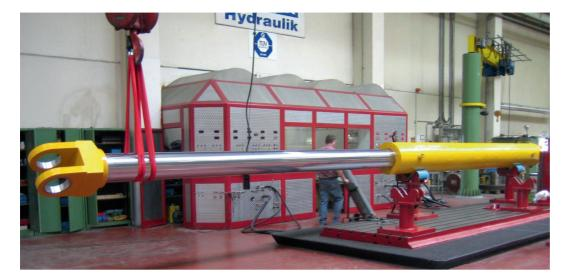
A typical application are for type GE...HS radial spherical plain bearings is use in mid-sized and large cylinders for maritime applications. The strict requirements for corrosion resistance make the use of special materials and seal designs necessary.
