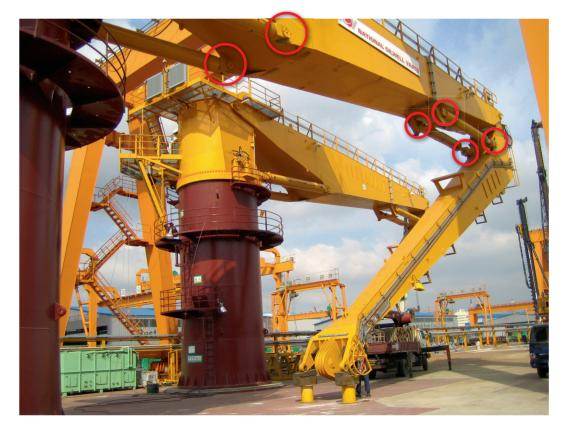
An example of the use of type GE...HS radial spherical plain bearings that has been successful for many years: HUNGER-hydraulic cylinders for ship and loading cranes.
